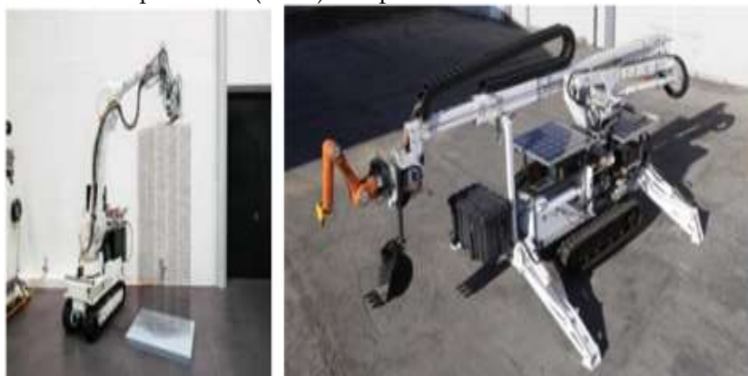
Pic. 2. Mobile self-propelled tracked printer
